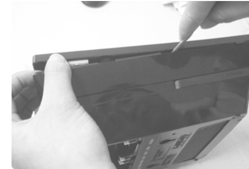
D.Keep on moving the blade to position of 60mm again, and press it, then open the position of lock
