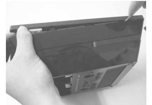
E.Keep on moving the blade to position of 60mm again, and press it, then open the position of lock.
