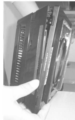
M.Loosen screws 3×6BM(2pcs) to remove plank of speaker
