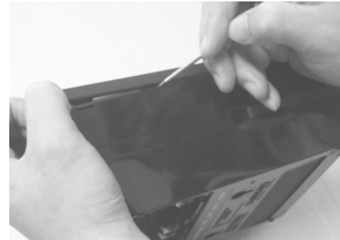
C.Keep on moving the blade (it's about 5mm width) to position of 45mm, and press it, then open the position of lock
